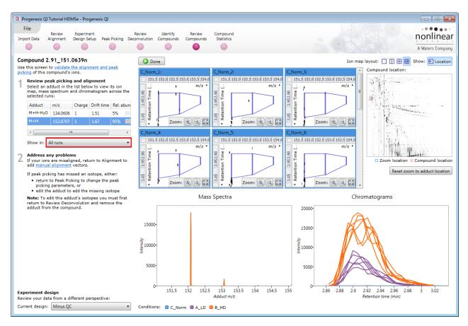
Use the lon map layout and zoom tools to set up the views as shown above. The multi-panels allow you to confirm the alignment across all the runs.
