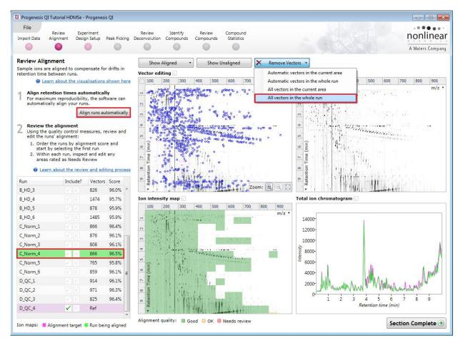
The alignment quality of this data set does not require any manual intervention so before going to the next section make sure you have Removed all manual vectors and re-performed the Automatic alignment. To do this for C\_Norm\_4 first select Remove 'All vectors in the whole run' and then click Align runs automatically.
