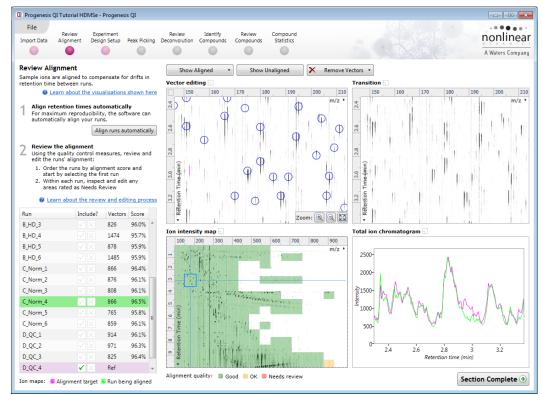
Using the **Simulated** miss-aligned example from the previous section to explain the review process for alignment, the alignment looks as below with a region of poor alignment (highlighted in red).
