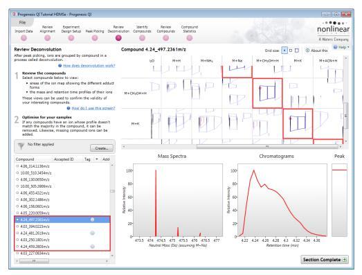
As an example to explore the posibility that **Compound 4.24\_497.2361's** sole adduct is M+Na try hovering over the detected peaks for the expected adducts. In this case when you hover over M+H as the possible second adduct you can see that although the chromatograms elute at the same retention time the mass
