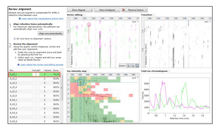
9. Repeat this process moving the focus from top to bottom on the **Ion Intensity Map** view the number you add is dependent on the length of gradient used and the severity of the misalignment. In many cases a single vector per alignment is all that is required to improve the performance of the Automatic Alignment
